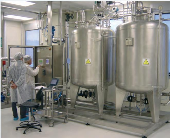
▲ CIP plant with control board on side machine with vertical tanks
