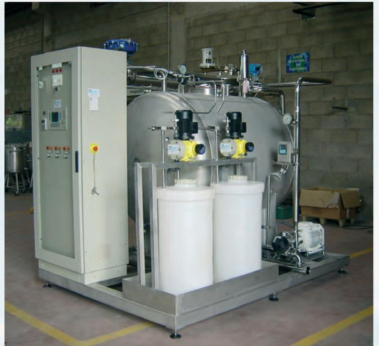
CIP plant with control board on side machine with orizontal tank ▲
