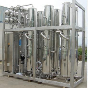
Distilliler mod. M-REM 2500 from 2.500 lt./h PED97/23/CE tested
