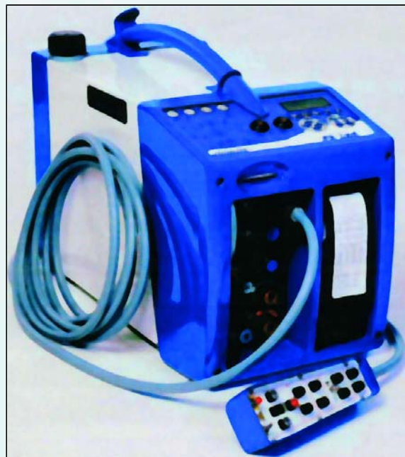
▼ Saldatrice orbitale con Report stampato Orbital welding machine with printed report
